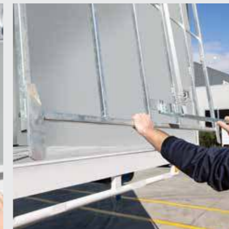
STEP 3: LOWER AND SMOOTHLY SLIDE GATE SIDWAYS
