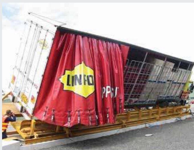
TILT BRIDGE TESTING - FULLY ENGINEERED AND APPROVED LOAD RESTRAINT
